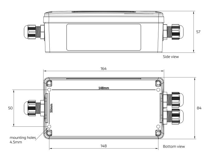
IP67 ABS field case fitted with 3 M16 cable glands Cable diameter: 4mm (0.16") to 7mm (0.27")
